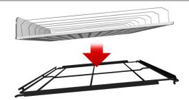
• FlexRoller installs onto (lays over) the cold vault wire shelves
